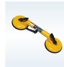
XP009 角度可调吸盘 Angle adjustable chuck 规格/SIZE : 可调 (Can adjust) 90°-270° 胶盘直径 (Rubber disc dia) 118mm 最大吸力/Max.suction : 35KG
